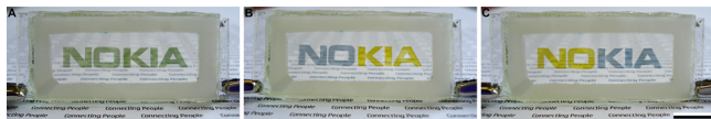
Figure 5. Photographs of an electrochromic supercapacitor device displaying color change upon charge and discharge. The letters “NO” form the double-gyroid structured top electrode and “KIA” the bottom electrode (scale bar: 1 cm). Both V_2O_5 electrodes have identical area. (A) Discharged green state at 0 V. (B,C) Charged state at \pm 3.5 V for reverse polarity with green/gray reduced and yellow oxidized electrodes. This device is still fully functional after six months.
