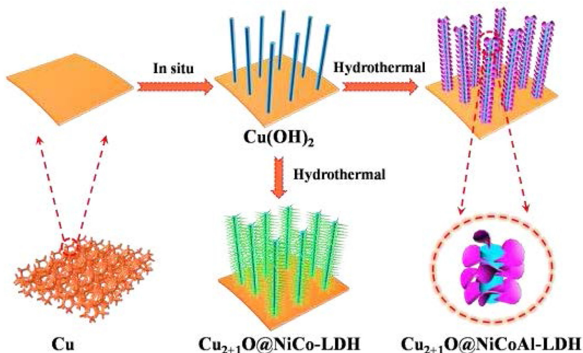
Fig. 1. Schematic illustration for the preparation of the \text{Cu}_{2+1}\text{O}@\text{NiCo-LDH} and \text{Cu}_{2+1}\text{O}@\text{NiCoAl-LDH} materials.
