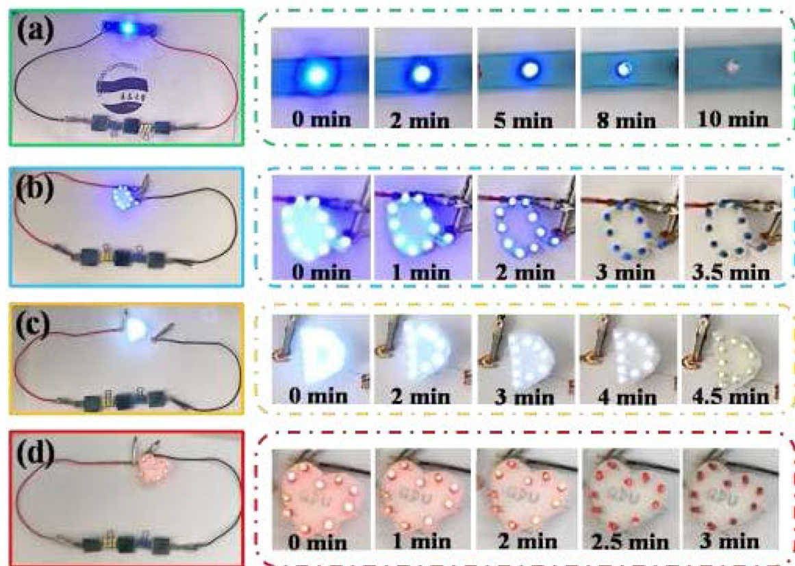
Fig. 8. Photographic images of the solid-state hybrid supercapacitors for lighting (a) the blue LED bulb, (b) the letter “Q” composed of 10 blue LED indicators in parallel, (c) the letter “D” composed of 10 yellow LED indicators in parallel and (d) a heart-shaped combination of ten red LED indicators connected in parallel. (For interpretation of the references to color in this figure legend, the reader is referred to the Web version of this article.)
