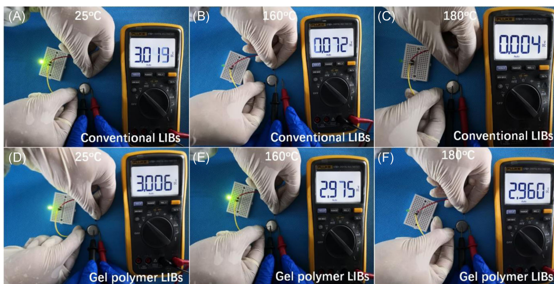
FIGURE 4 Optical images of (A–C) the conventional and (D–F) gel polymer coin-type full cells, connected to a voltmeter and a green light-emitting diode (LED). Coin-type full cells (A,D) before and after thermal treatment at (B,E) 160°C and (C,F) 180°C for 1 h. LIB, lithium-ion battery
